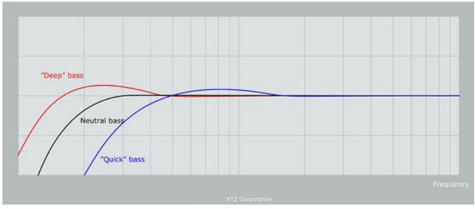
This schematic picture (which does not shown actual measured curves) elucidates the different sonic characteristics of the bass frequencies.
