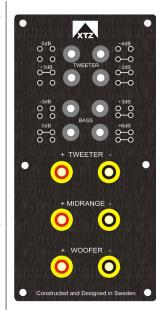
Note! Make sure that all jumpers are connected. A loose jumper may cause a short-circuit if they jam between the terminals.
