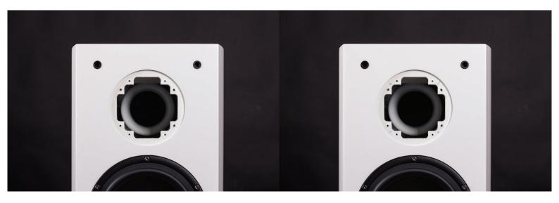
When the old tweeter is removed it is possible to place the Beryllium tweeter, be sure that the holes are in a straight line horizontally or vertically, then use a pencil to mark where the holes should be.
