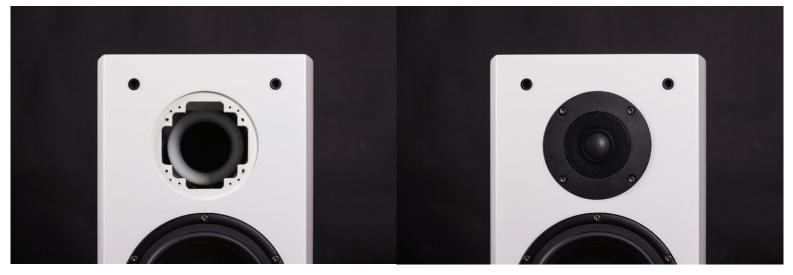
Use a 2 mm drill, and be sure the drill is orthogonal to the baffle when drilling. To make a tight seal around the new tweeter ensure the old holes does not have any material poking out, Use a countersink or larger drill to remove peaks. As long as the surface is flat/smooth behind the new tweeter, the seal is airtight enough.
