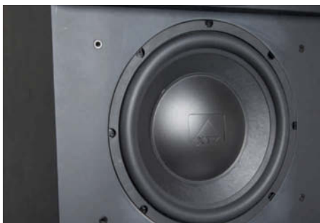
The three front panels are mounted with four screws each, and happily, there are threaded inserts in the front baffle.
