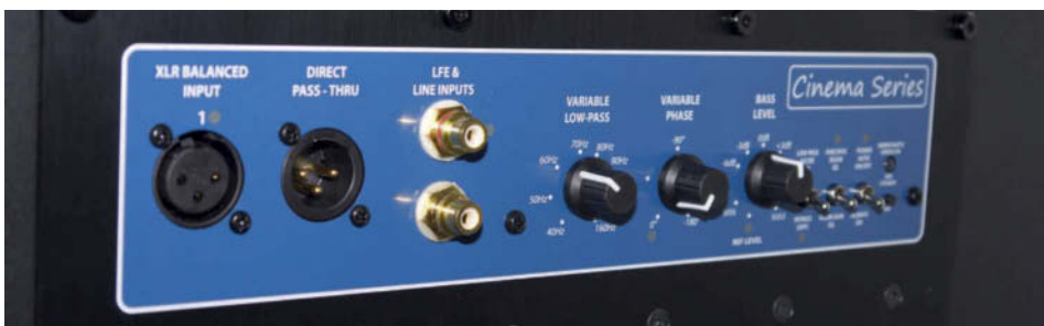
Balanced input, yes please! Knobs for crossover frequency, volume and phase. Switches for low-pass filter on / off (set to off if you want to give your amp full control of sub 3x12), Room EQ and choice if the power should be automatic or always on. At the far end is a button labeled "pair", and it has no function. Right now, anyway. Olle at XTZ says it "might" be used with a later update, and we're guessing that they are thinking of doing sub 3x12 wireless.
